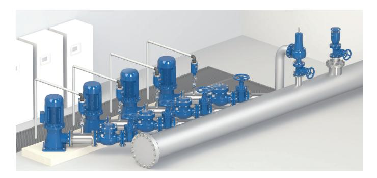
**Pressure reduction valve station.** In this second layout Gemina is installed downstream of a pressure reduction valve station to prevent in any case rise in pressure on the main line. The installation also includes the pressure reducing valve CSA XLC 310/410, a by-pass for maintenance and anti-surge combination air valves FOX or LYNX 3F AS upstream and downstream.
